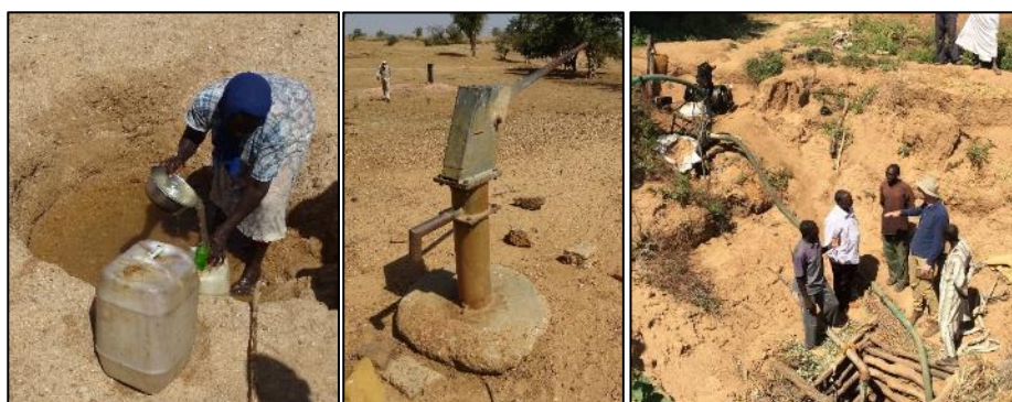
Figure 11. From left to right: (1) Scoop hole; (2) Hand pump; (3) Motorized pump in hand-dug well.
